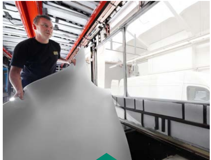
HANNO manufactures die-cut foam parts for noise protection and thermal insulation in trains and trams.
